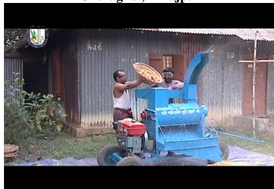
Fig 5.18 Shallow machine operated maize sheller Joydebpur, Gazipur
