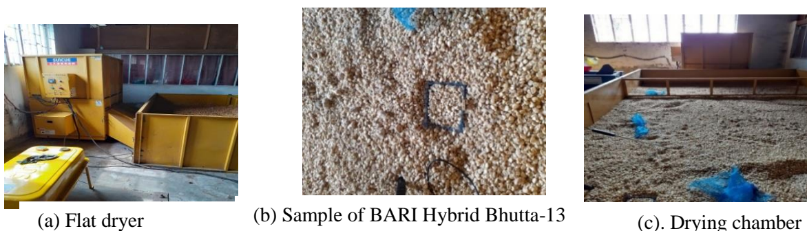
Fig.1. Pictorial view of the flat bed dryer and dried grains.
