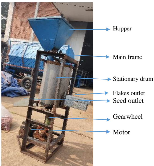
Fig. 1. Chilli seed separator.
