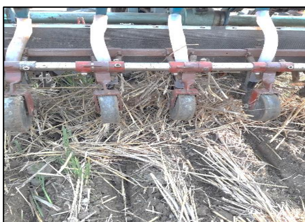
Fig 17. Residue stuck in furrow opener without attachment of residue clearing device.
