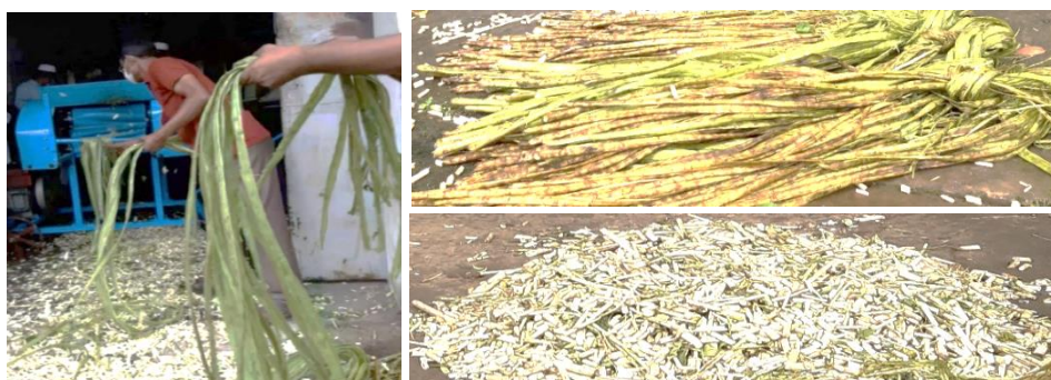
Fig. 15. Jute ribbons in full length and broken jute sticks extracted by jute decorticator.
