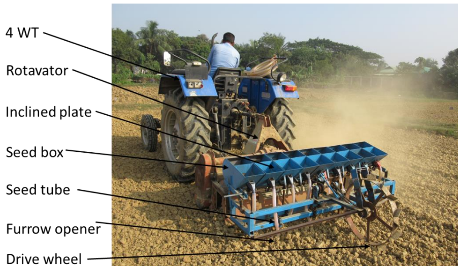
Fig. 3. Major functional components of the fabricated 4WT operated seeder.
