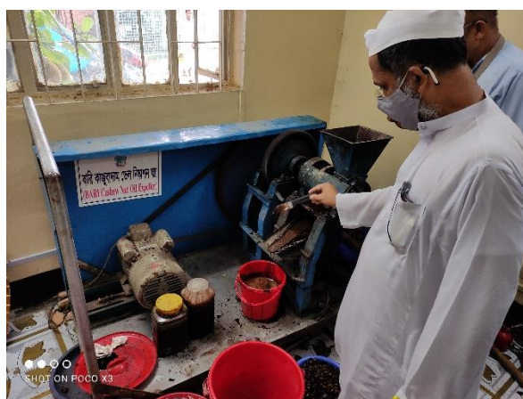
Fig. 3. Performance test of the oil expeller with cashew nut shell.
