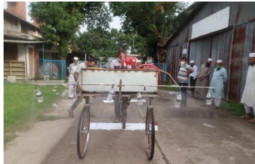
Fig 9. Measurement of missing and overlapped spraying area percentage.
