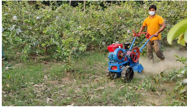
Fig 2. Field performance evaluation of orchard weeder in a guava orchard.
