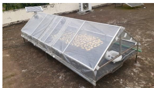
Fig 5. Solar tunnel dryer with heating system.
