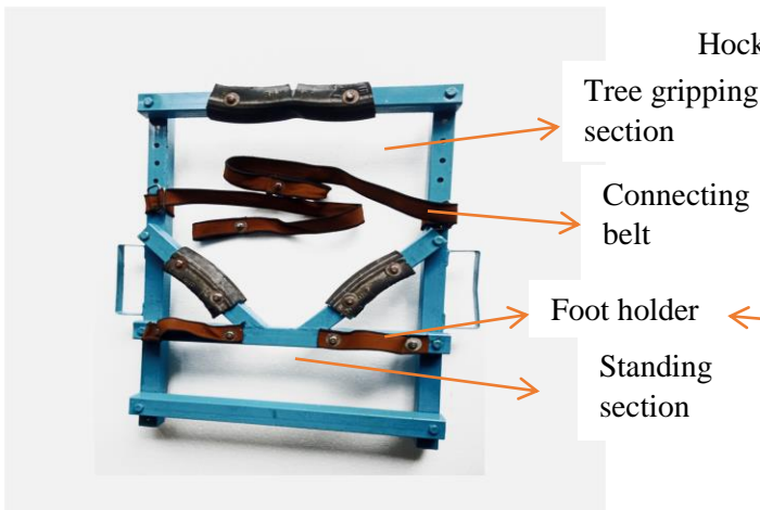
Fig. 3. Lower frame of the previous climber.
